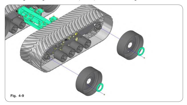
8. Using a safe lifting device rated at 600 lbs., remove front and rear outside idler wheels. Retain parts and hardware for reassembly. (Fig. 4-9)
