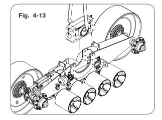
14. Place the new trunnion assembly into track frame with the grease fittings facing up as shown in Fig. 4-14.
