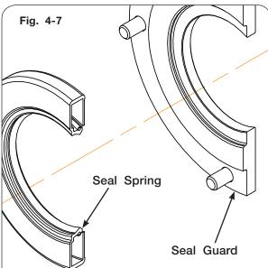
Be sure spring side of the seal faces outside of hub towards the seal guard.
